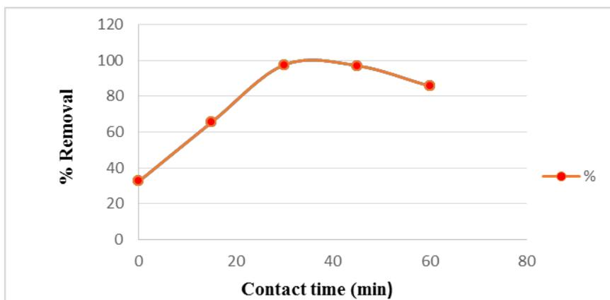
Figure 2: Effect of contact time on percentage removal of Nickel (II).
