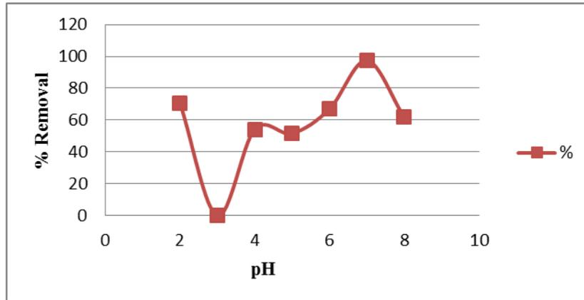
Figure 3. Effect of pH on percentage removal of Nickel (II)
