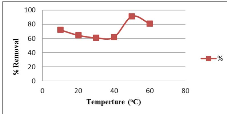
Figure 4. Effect of Temperature on percentage removal of Nickel (II).
