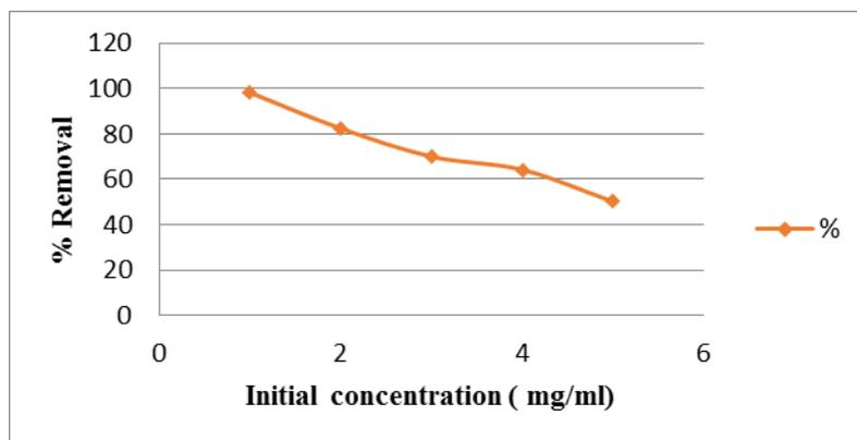
Figure 5: Effect of concentration on percentage removal of Nickel (II).
