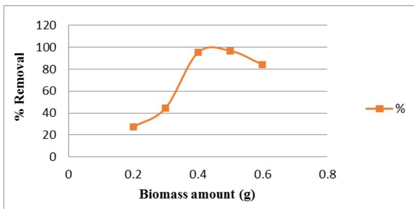
Figure 1: Effect of biomass on percentage removal of Nickel (II).
